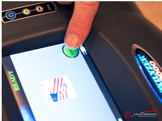
Figure 4 - The touchscreen interface in the test unit had calibration issues and proved to be a frustrating interface to the instrument's operational sequencing.
